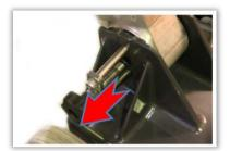
8. Remove the handle by taking it out of the cradle on the motor base frame and reposition the centring pin in the holder on the handle.
