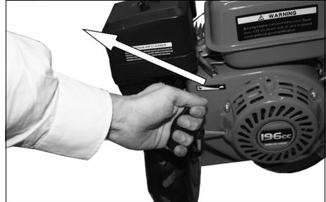
6. Once the engine starts, move the choke to the 1/2 way position.
